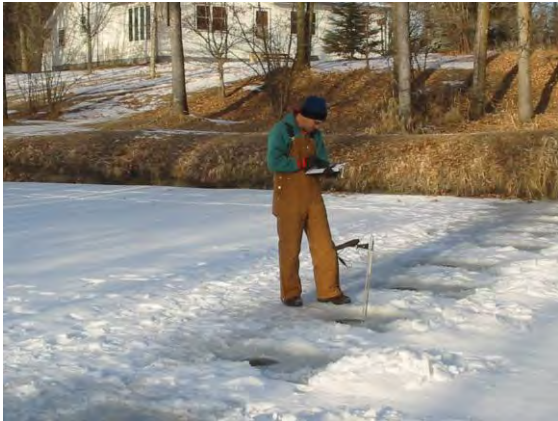
Measuring flow beneath ice
