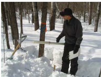
Establish base weight of empty sampling tube
