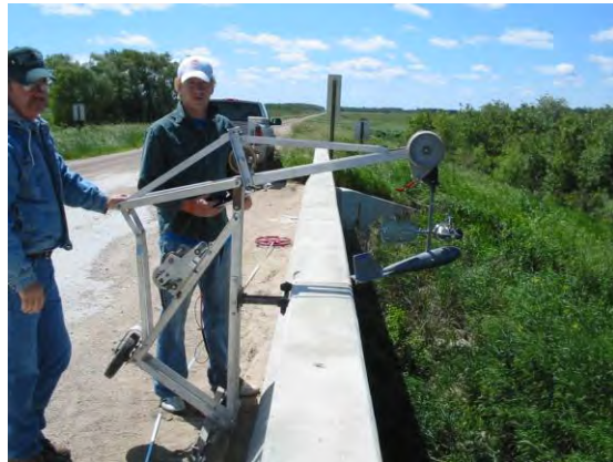
Measuring flow with bridge crane
