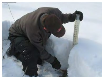
Obtaining snow depth and core sample
